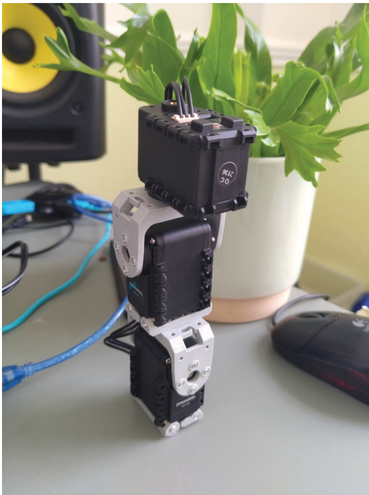
Figure 3. One of our robots, created from three ROBOTIS servo motors coupled with standard fixings, creating three degrees of freedom. (Photo by Alex McLean)
