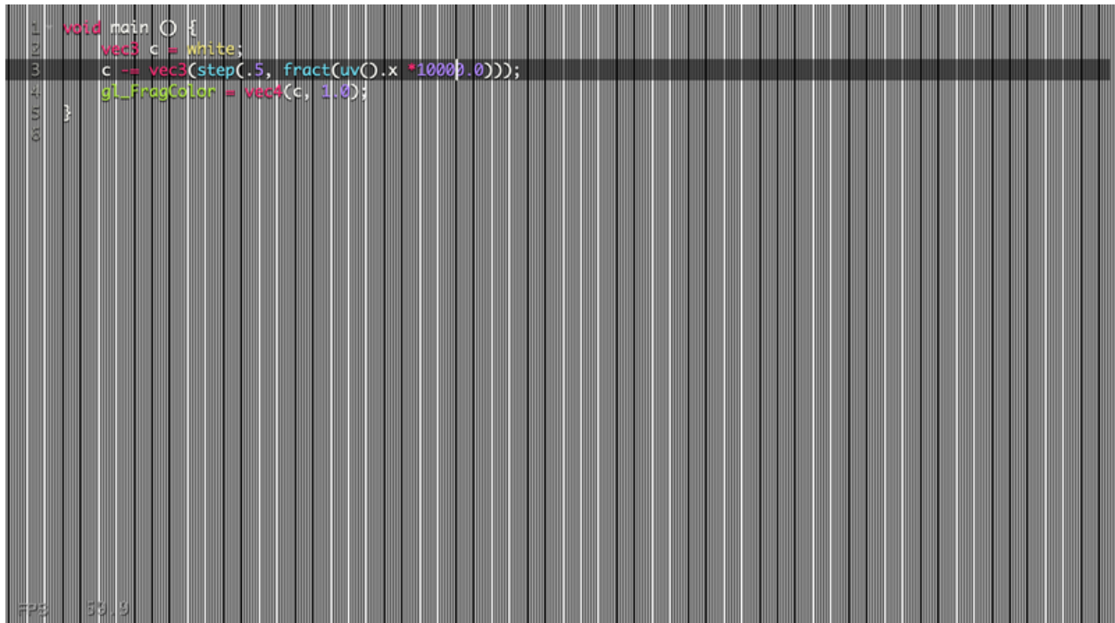
Figure 4 Example of digital aliasing in GLSL.
