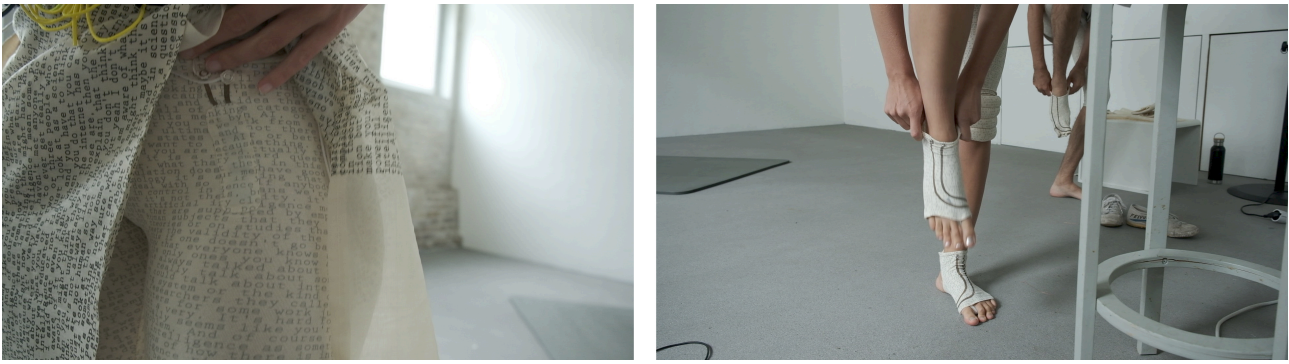
Figure 1: Left: E-Textile pressure sensor embedded in undergarment; Right: E-Textile pressure sensor on socks measuring the foot pressure against the floor. Both are from the early prototype costumes.
