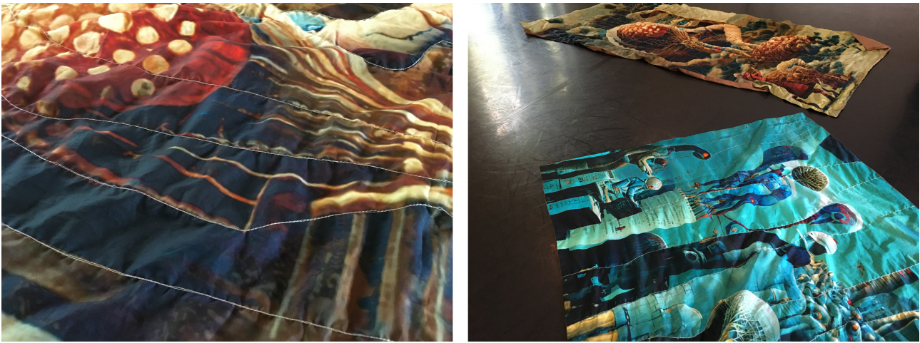
Figure 2: Left: Conductive thread embroidery as capacitive touch sensor on a fabric; Right: Large-scale digital printed fabric with AI generated images
