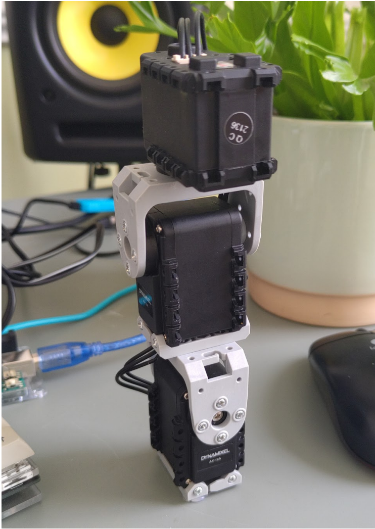
Figure 2: One of our robots, created from three ROBOTIS servo motors coupled with standard fixings, creating three degrees of freedom.
