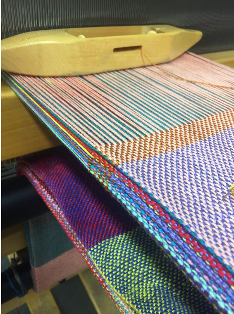
Figure 9 Edge detail of continuous weft technique on loom
