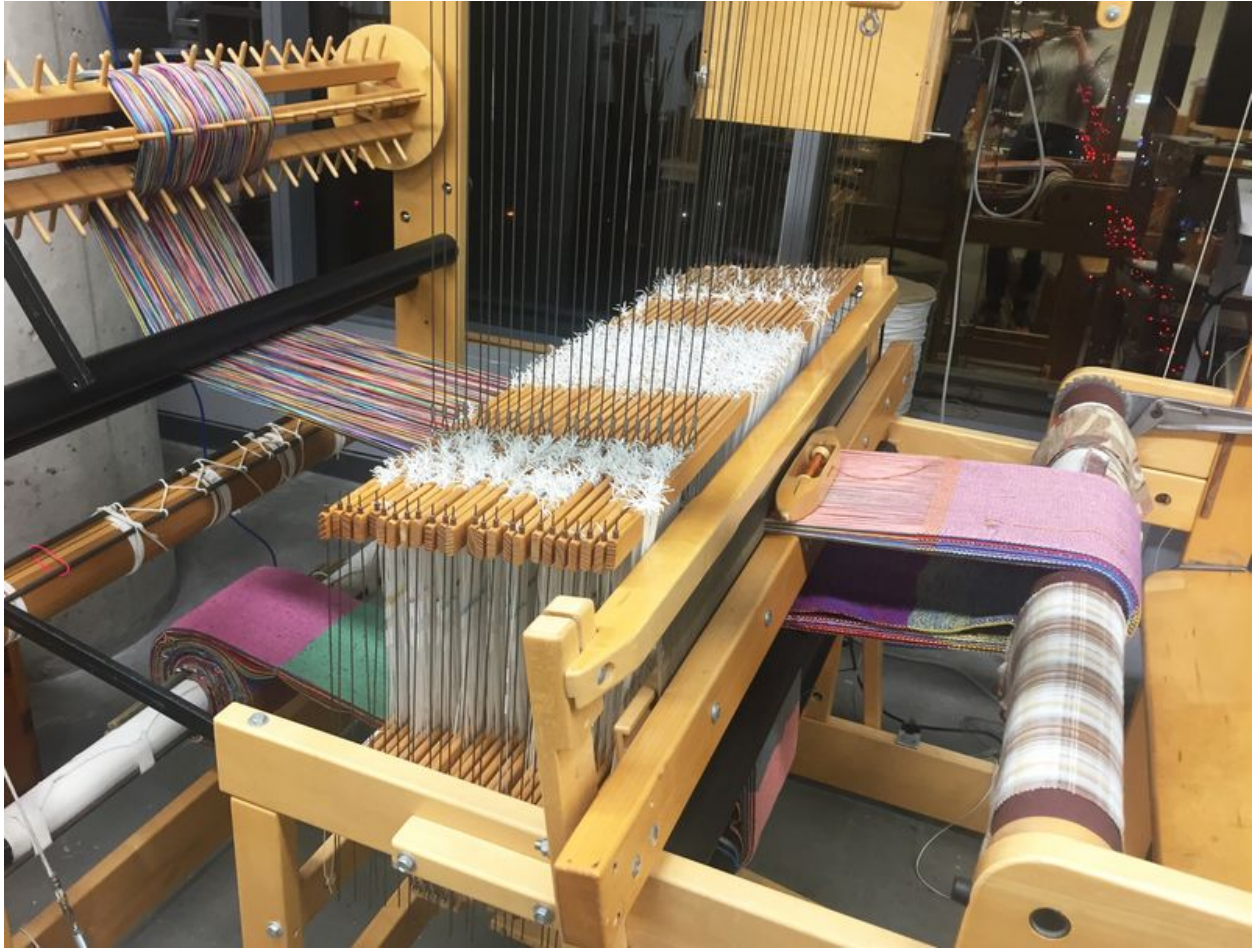
Figure 11 Weaving on 24-harness dobbie loom
