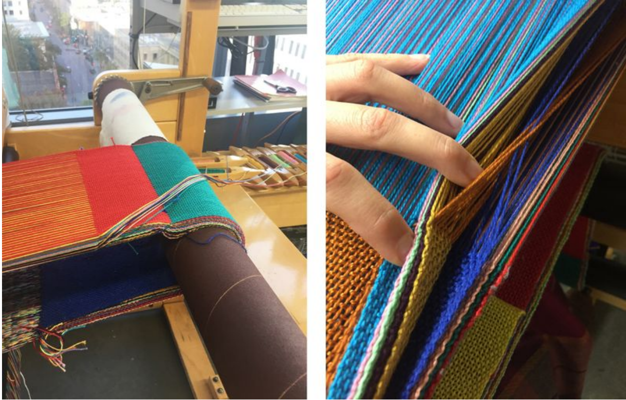
Figure 7 Weaving stacked layers with multiple-weft technique
